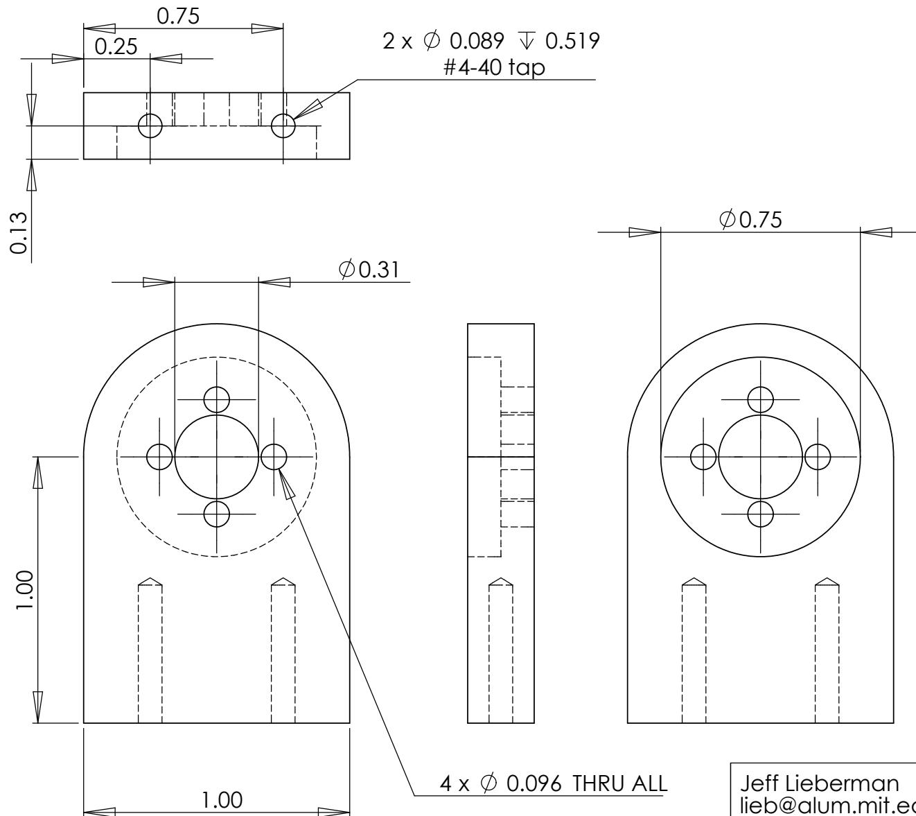
Note: Final dimensions of motor mounting (plunge size/depth, hole pattern) to be specified soon - still specifying final motor. No general details will change, only specifics. Looking for preliminary quote.
